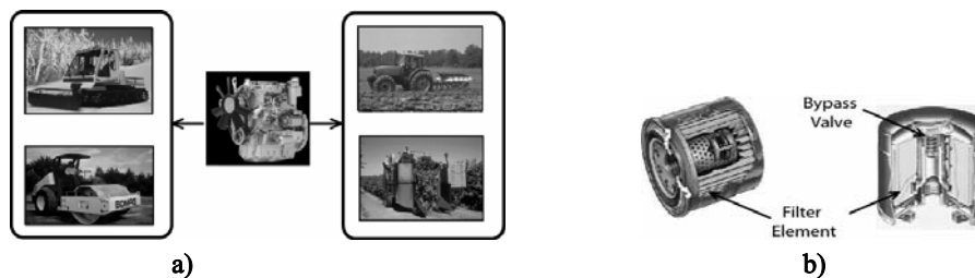
Figure 4. (a) Applications of a one engine model (b) Oil filter cutaway
