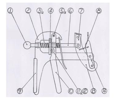
Figure 6. A machine for tightening brake cables
