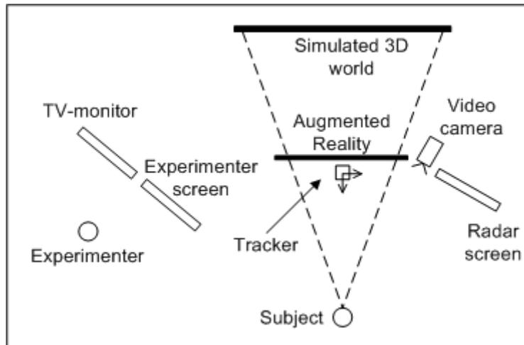
**Figure 1. Schematic view of the experiment setup, as seen from above**
