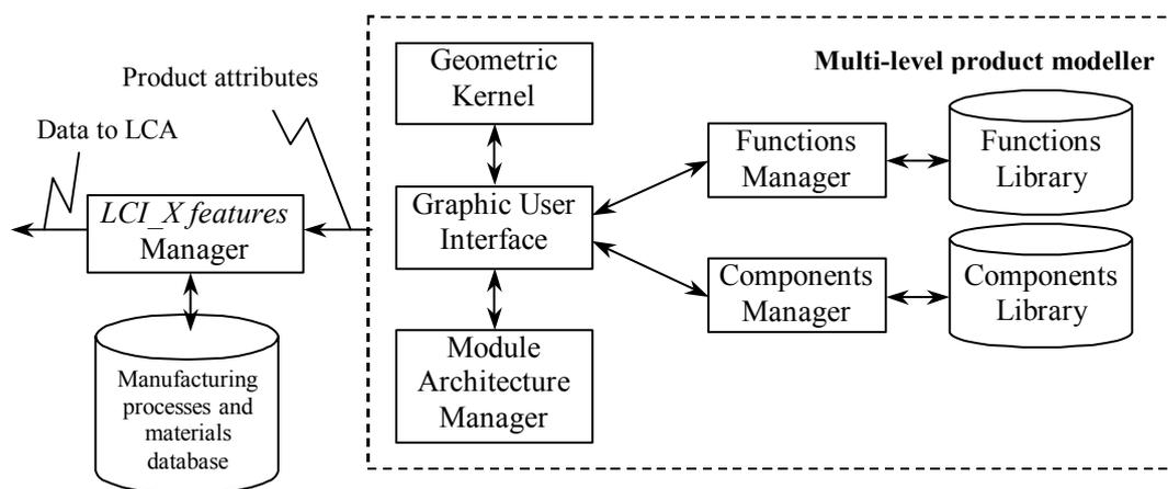
Figure 4. Main modules of the software system architecture
