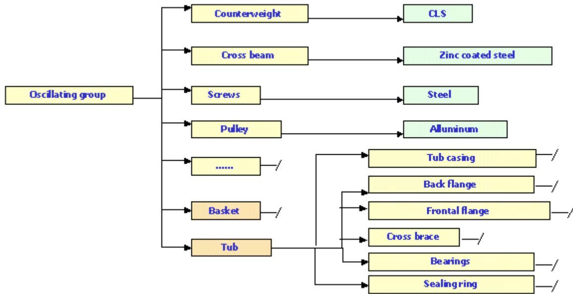
Figure 6. Oscillating sub group components and related materials
