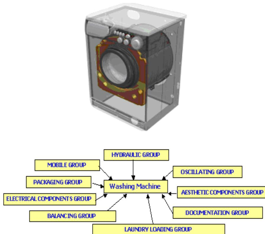
Figure 5. CAD model and meaningful washing machines groups useful for LCI definition
