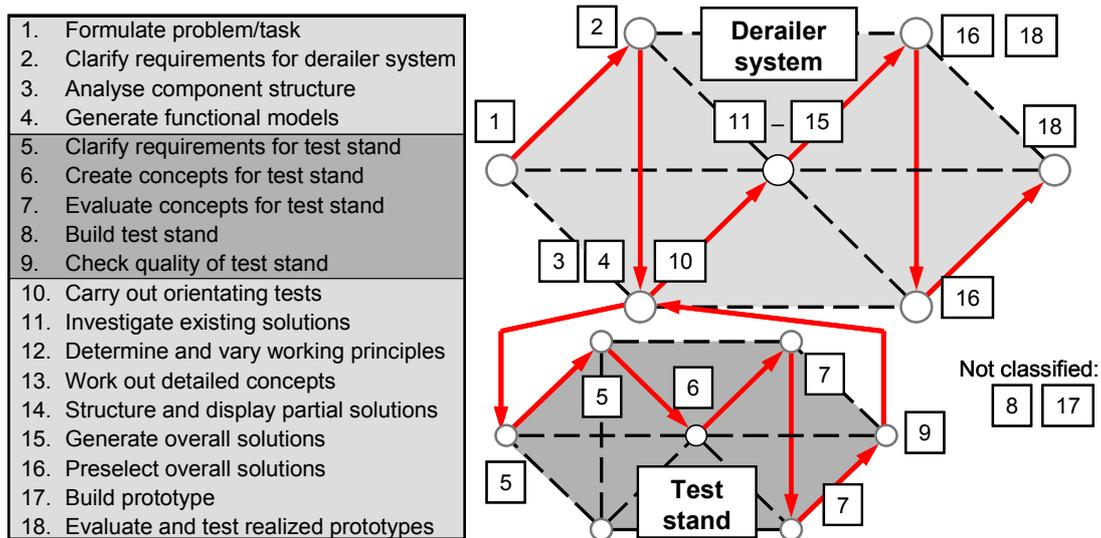
Figure 5. Process pattern (on superordinate level) in the case study “derailer system for recumbent bikes”
