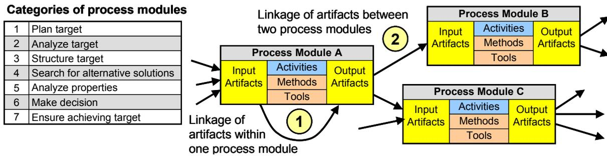
Figure 3. Linkage of artifacts within the network of process modules
