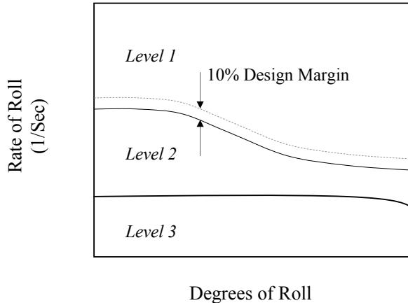
Figure 2.3. Handling Quality (quickness of roll) and design margin [10]
