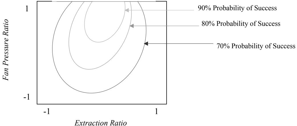
Figure 2.2. “Slicing” of CDF’s to Create Probability Contours [9]
