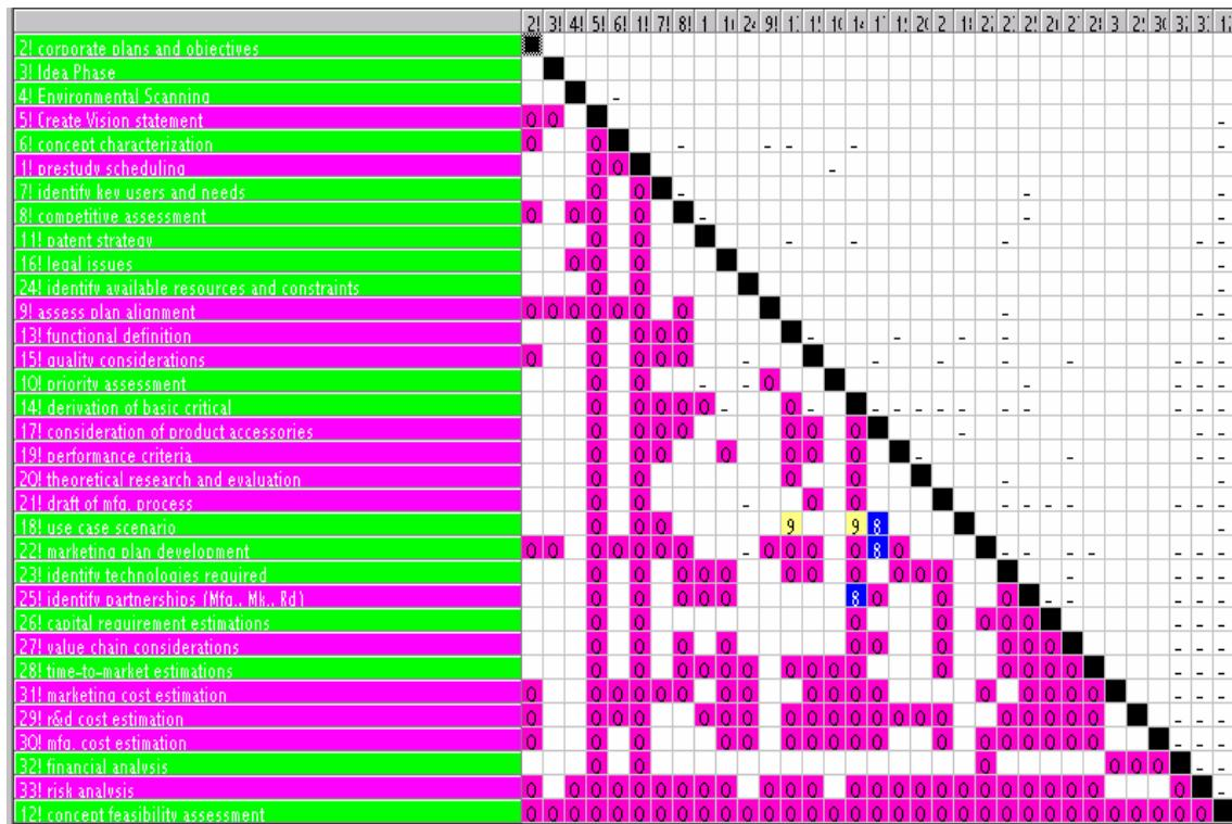
Figure 4: Banded view of the sequenced product concept phase as outputted from the PSM 32 software.
