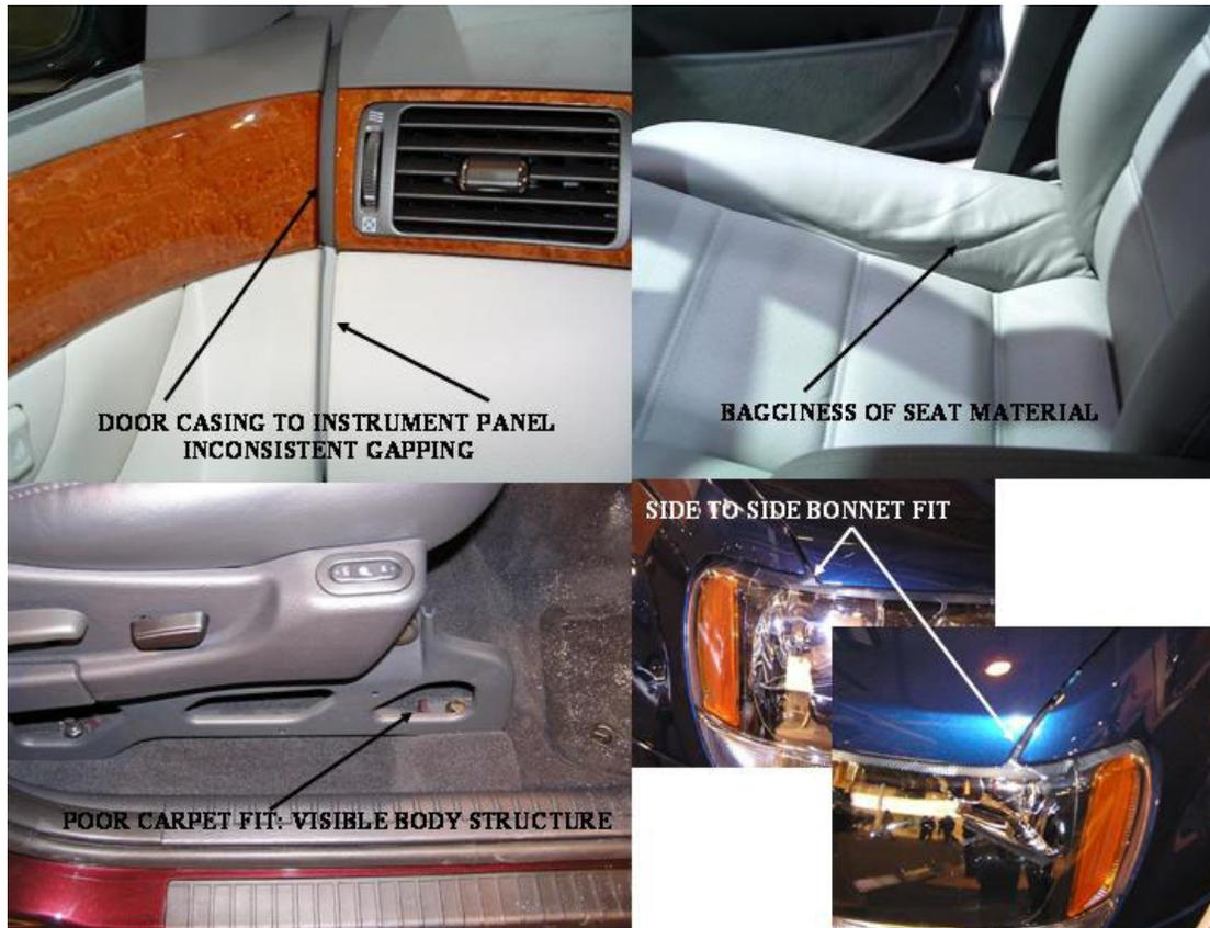
Figure 2: Poor Examples of Craftsmanship Execution
