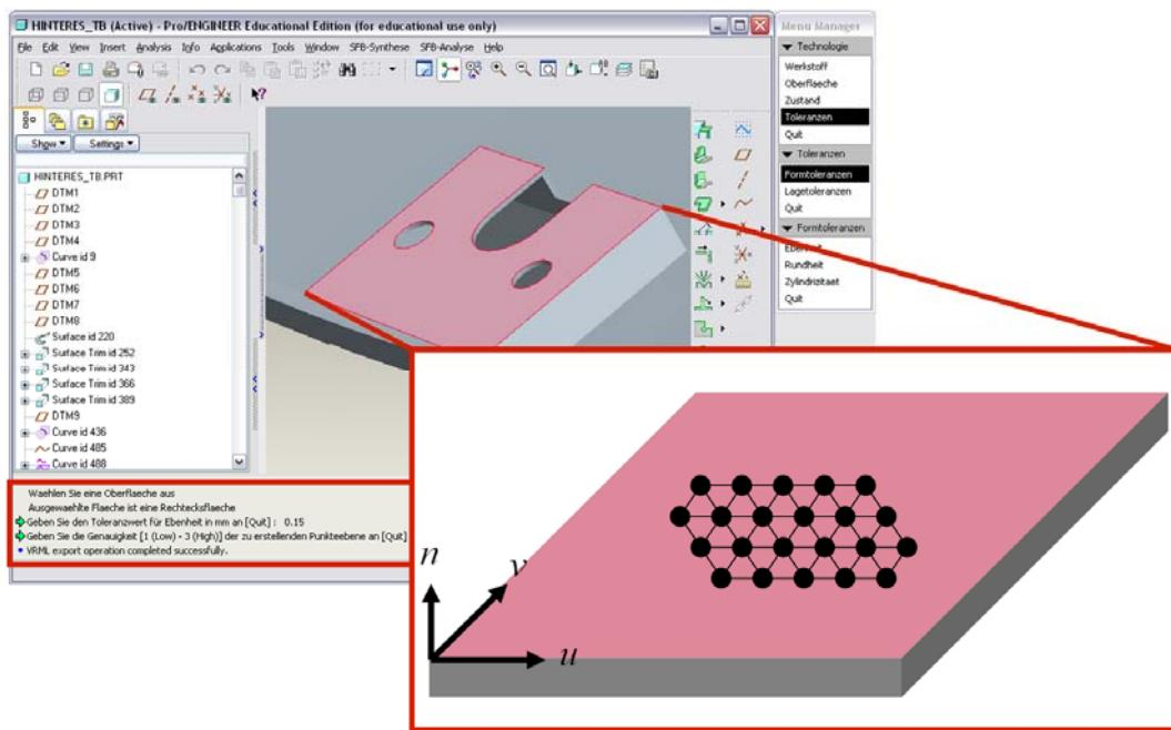
Figure 4. Tolerance definition and model preparation inside the CAD system
