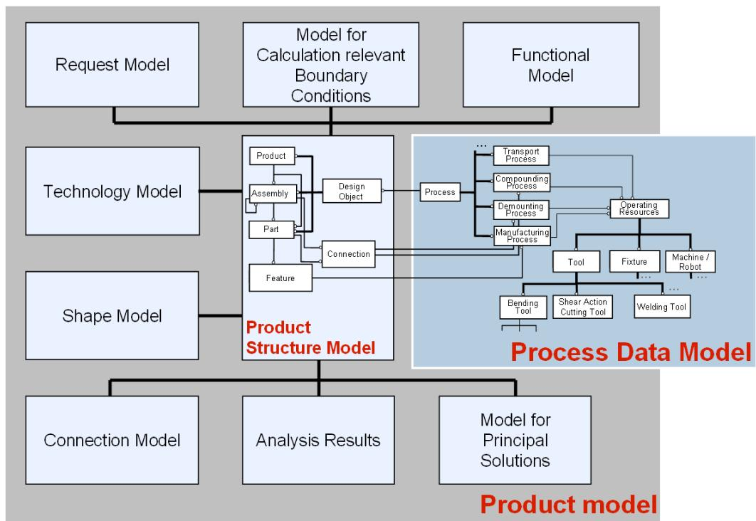
Figure 3. Structure of the hybrid data model of the engineering workbench
