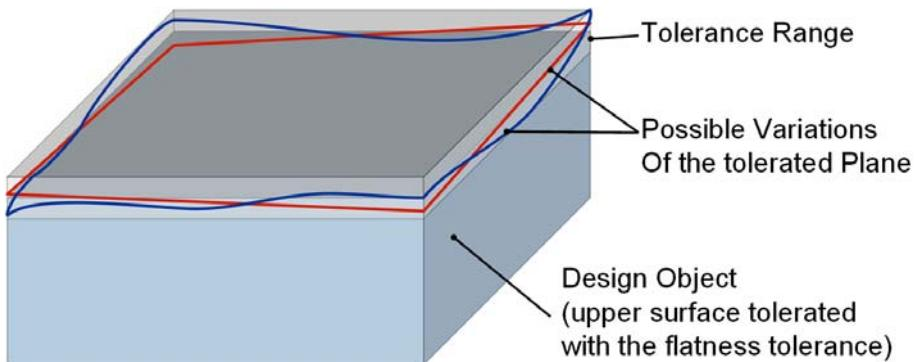
Figure 5. Tolerated cuboid and possible shape variations of the tolerated plain
