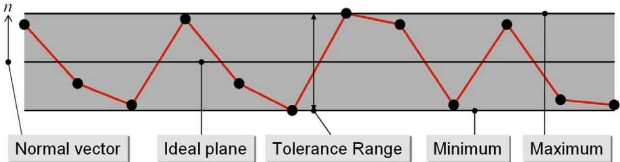
Figure 6. Side view of a random simulated shape variation of the tolerated plain
