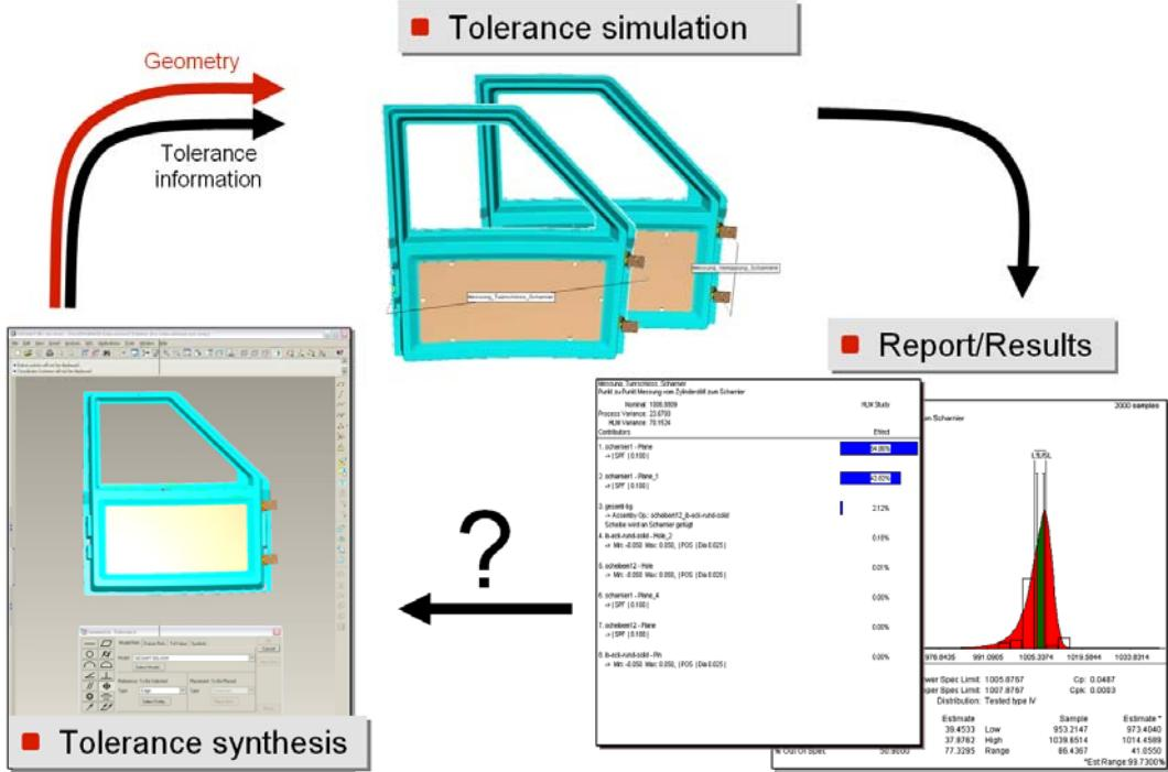
Figure 2. Process of a common tolerance simulation and analysis procedure
