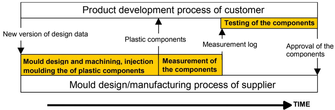
Figure 1. One iteration loop triggered by a new design document version.
