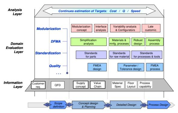
Figure 1. The general concept of DFX Platform
