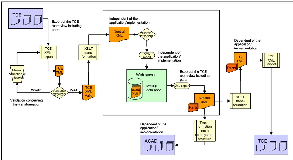
Figure 4. Product data exchange via the internet platform
