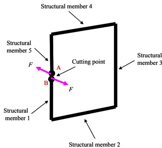
Figure 4. Structural model of the static force loop
