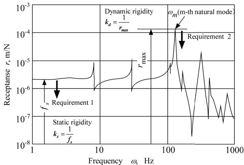
Figure 1. An example of frequency response at the cutting point of a machine-tool model
