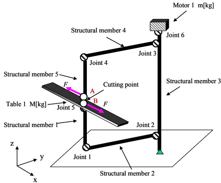
Figure 3. Framework model of a milling machine
