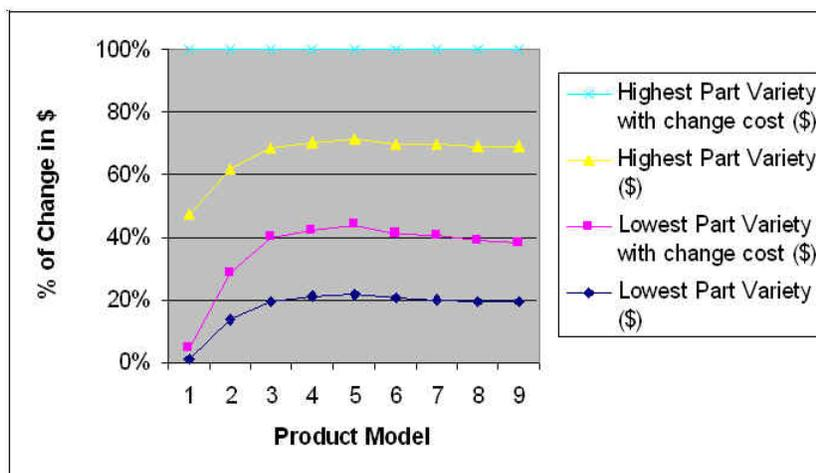
Figure 5. Cost Impact by Part Variety Level on the product models
