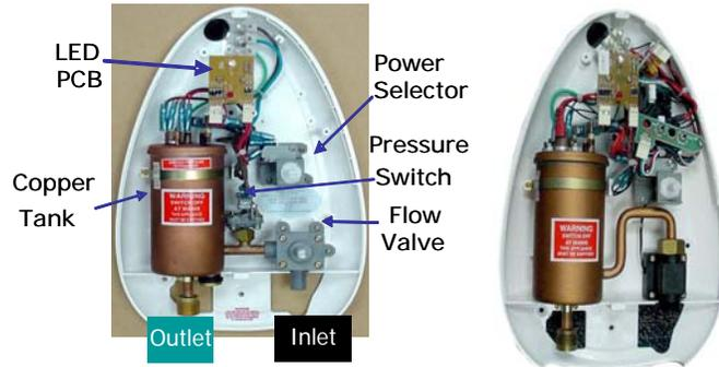
Figure 3. Two models of a family of Instantaneous Water Heaters
