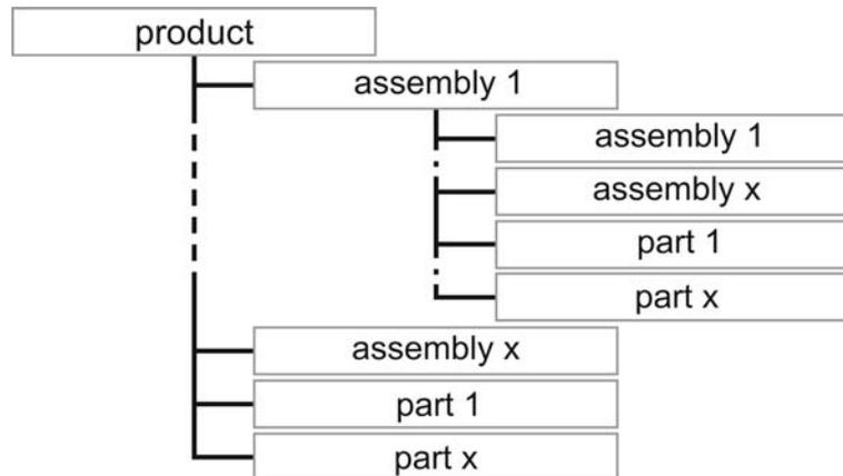
Figure 1. General component-oriented product structure
