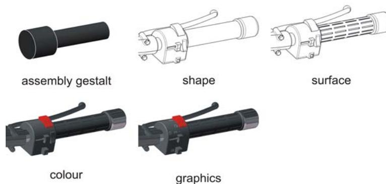
Figure 3. Assembly gestalt, shape, surface, colour and graphics of a motorbike hand grip
