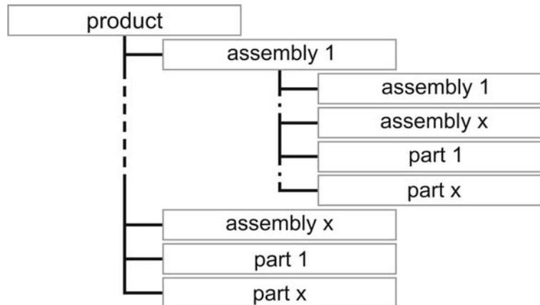
Figure 1. General component-oriented product structure
