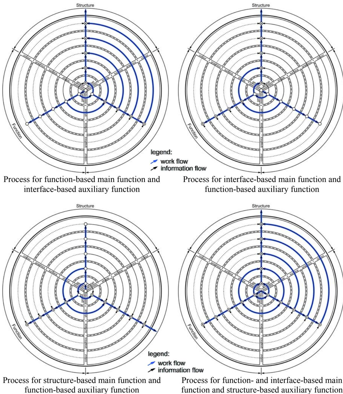
Figure 8. Adaptive product development process for main and auxiliary function
