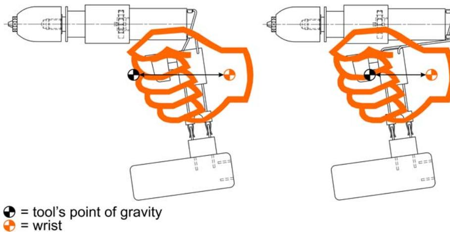
Figure 7. Point of gravity with different assembly gestalts of a power drill
