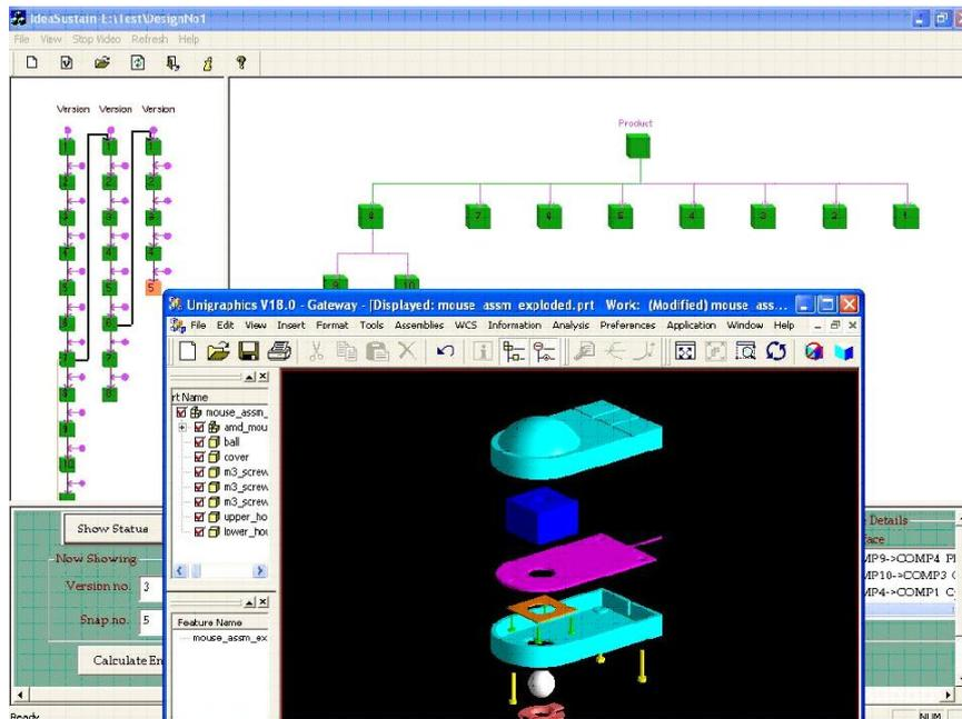
Figure 16 Product model in CAD software
