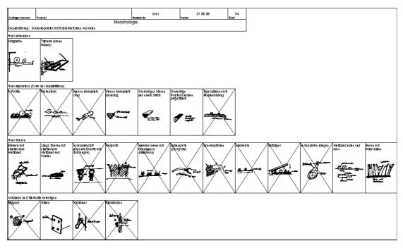
Figure 12. Morphological matrix of the pipe&tube holder
