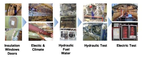
Figure 3. Equipment installation and test of fuselage systems
