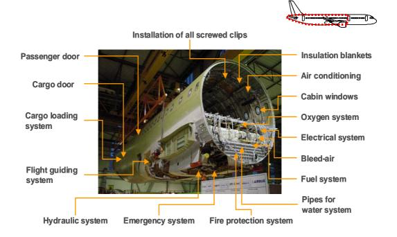
Figure 4. Equipment installation work packages for single aisle aircraft
