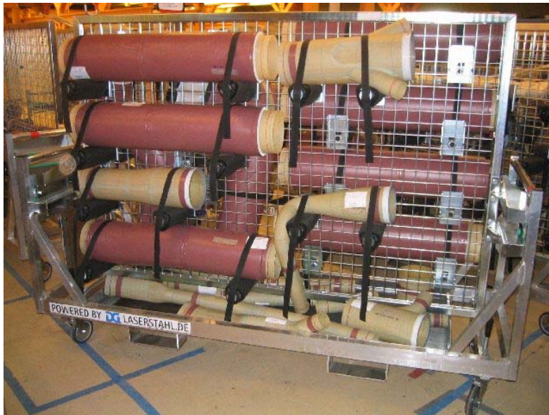
Figure 9. Pipe & Tube Distribution Unit with flexible adjustments for various types of pipes
