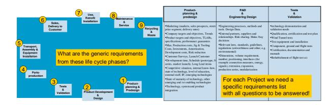
Figure 11. Product life-cycle phases and checklist for the systematic capturing of requirements
