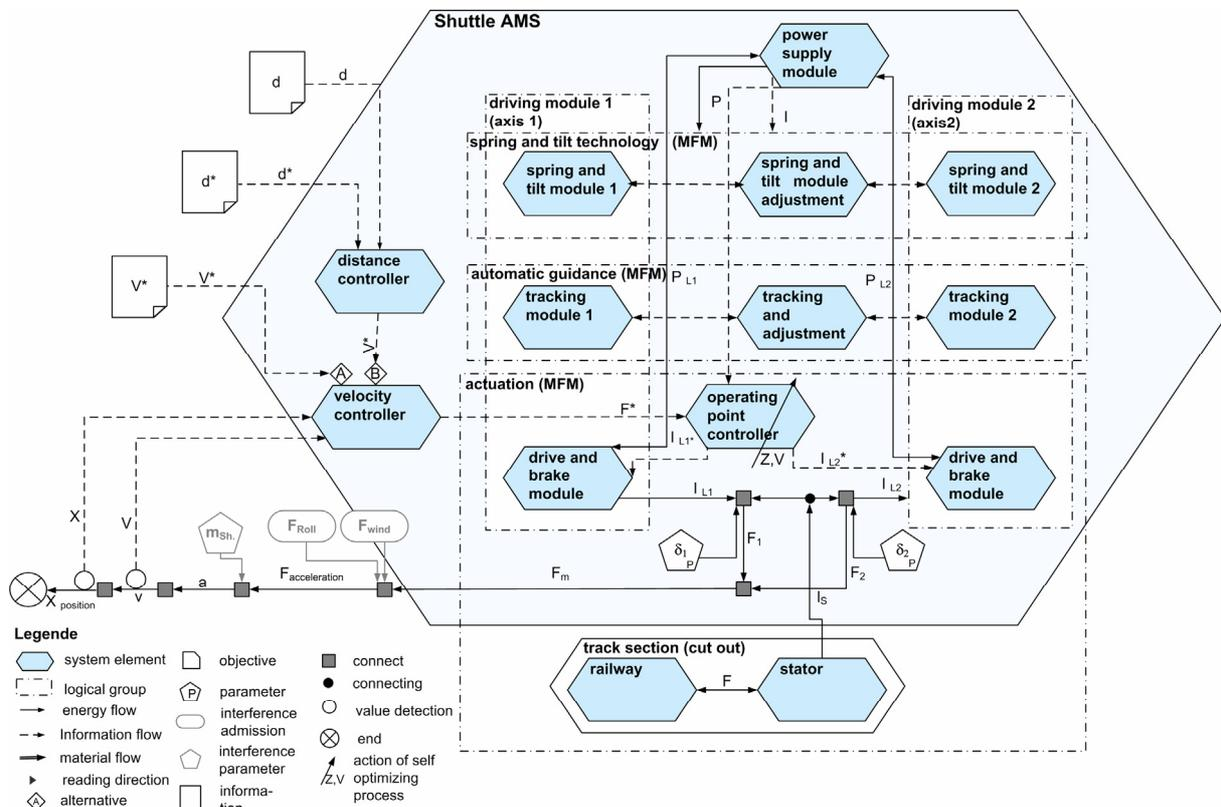
Figure 4. Active structure of a shuttle
