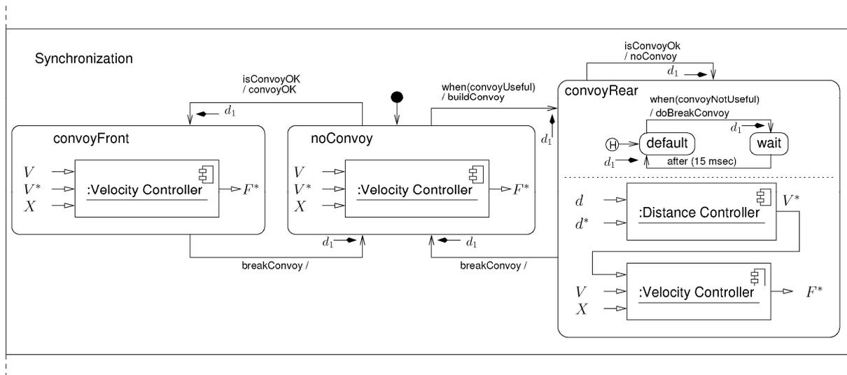
Figure 7. Extract of the Hybrid Reconfiguration Chart of the Shuttle software component
