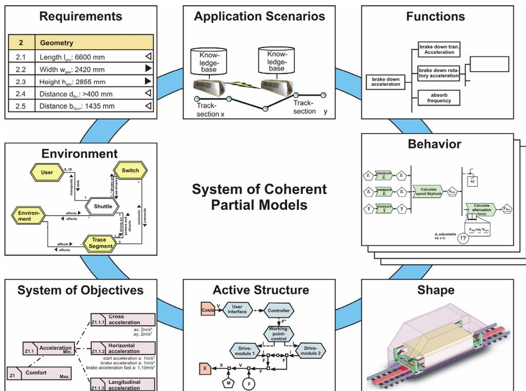
Figure 3. Coherent system of partial models for describing the principle solution of a self-optimizing system
