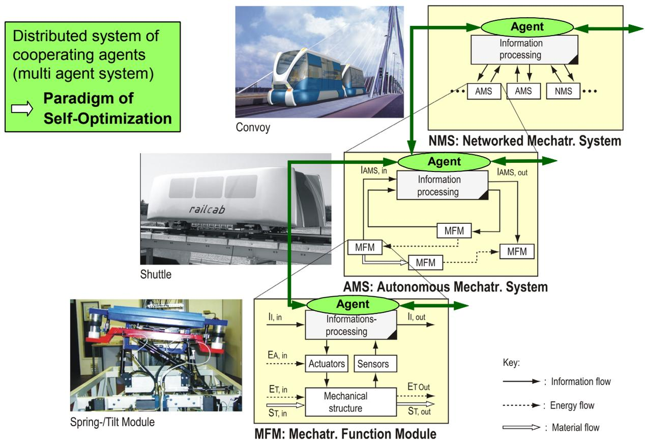
Figure 2. Hierarchical structure of mechatronic systems (according to Lückel [2])
