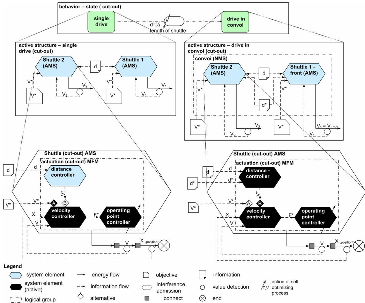
Figure 5. Relevant data in the principle solution for software design
