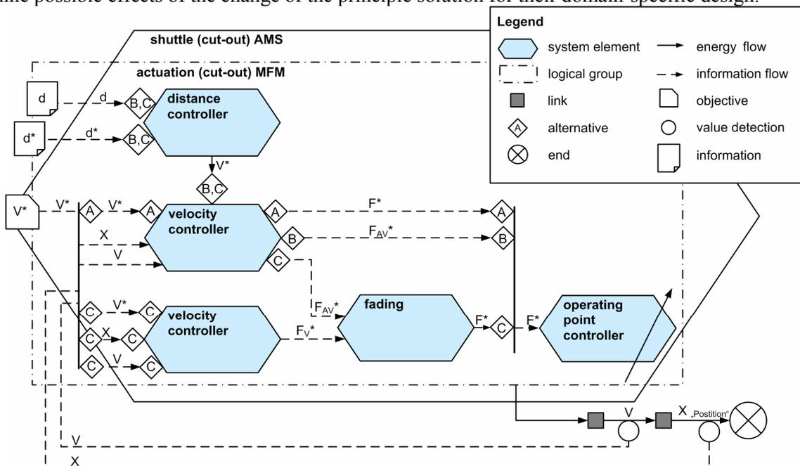
Figure 9. Addition of the fading functions in the active structure
