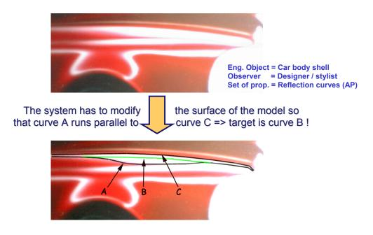
Figure 7. Shape Modification by Defining/Specifying Target Reflection Curves
