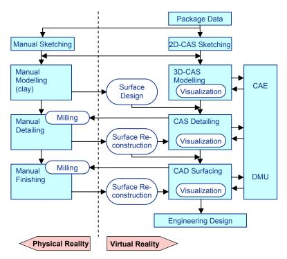
Figure 1. Generalized Aesthetic Design Workflow [1]
