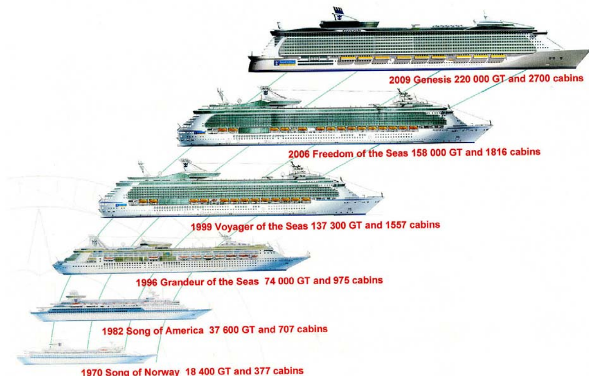
Figure 1: There has been significant growth in the size of the ships. The “Genesis” which is now under construction is almost 12 times bigger than “Song of Norway” from 1970. However the design and building time is not multiplied to tenfold – if the technical complexity is taken in calculations the calendar time needed in building are something between the same and doubled. [Picture and data: Aker Yards]
