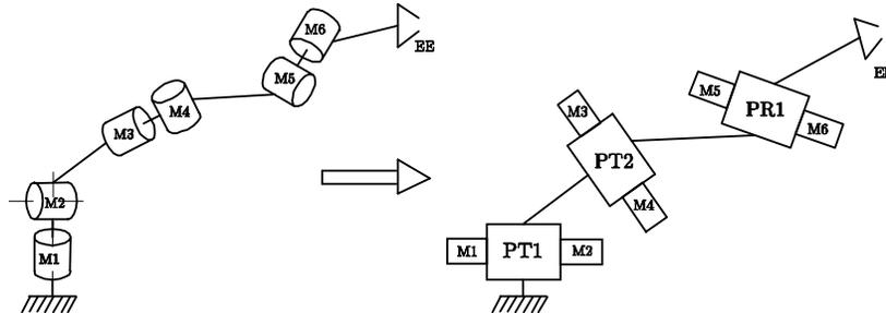
Figure 2. Proposed 6-dof hybrid manipulator
