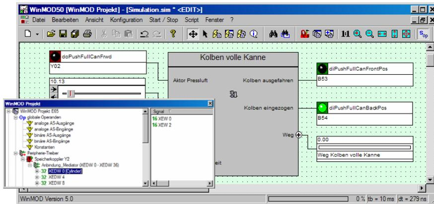
Figure 14 Cylinder in WinMOD
