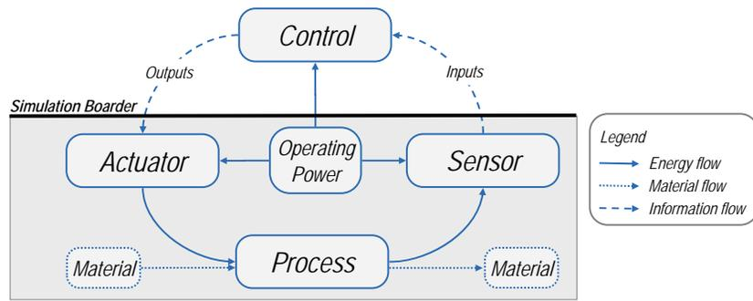
Figure 3 Principal setup of a mechatronic system
