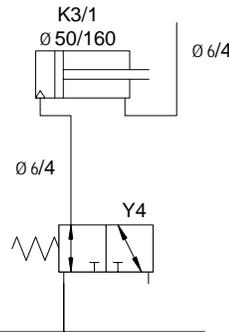
Figure 10 Cylinder in a pneumatic scheme
