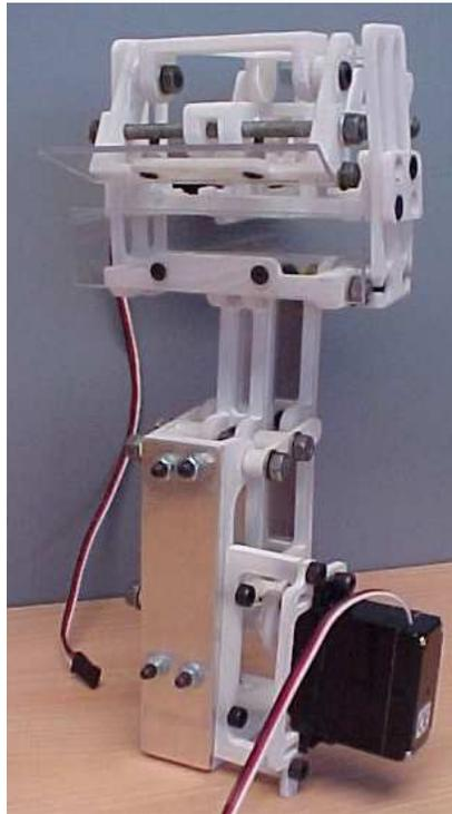
*Figure 11. Early folding mechanism prototype*
