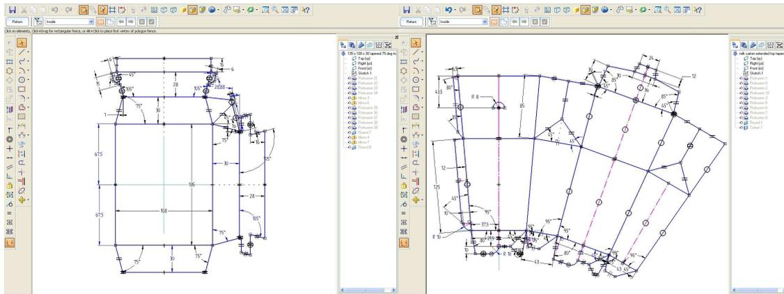
*Figure 4. Constrained parametric nets created within a commercial CAD system showing corner gussets (left) and gable top (right)*
