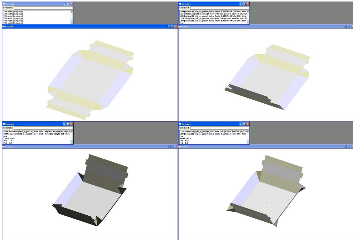
Figure 7. Origami tray shown flat (top left), with folds resulting from a single ground line rotation (top right), four simultaneous ground folds with gussets forced inwards (bottom left) and outwards (bottom right).
