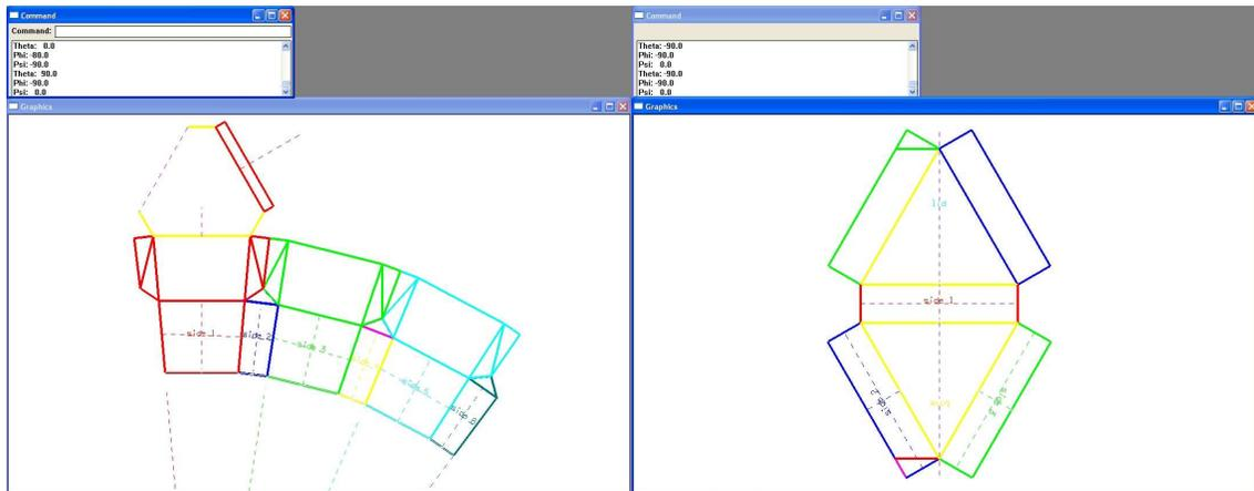
Figure 6. Generic carton simulation showing carton net for six sided gable top skillet (left) and triangular carton (right)
