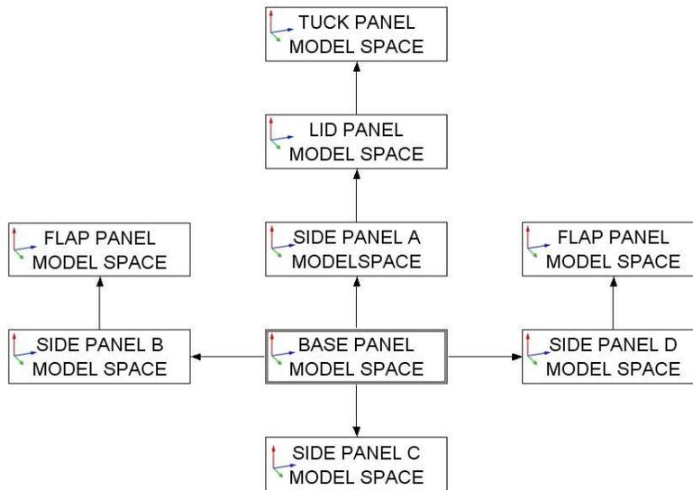
Figure 2. Model space arrangement in the origami model
