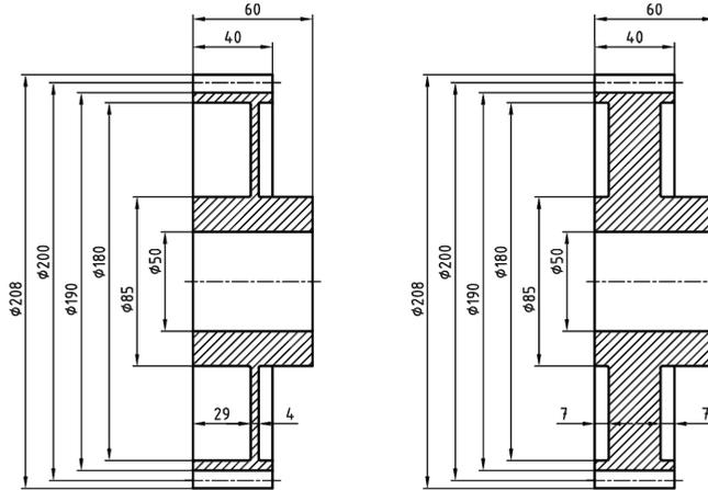
Figure 2. A pair of spur gears
