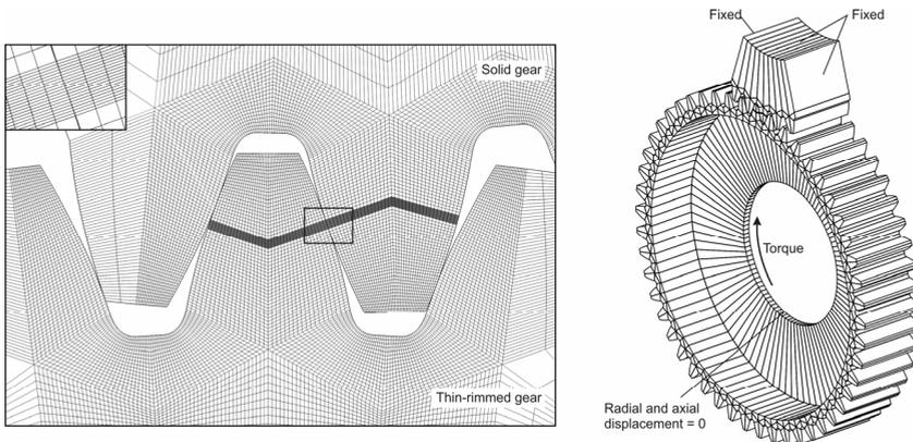
Figure 3. Model used in FEM analysis along with refined mesh detail
