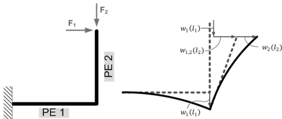
**Figure 8. Bending of profile-structures**
