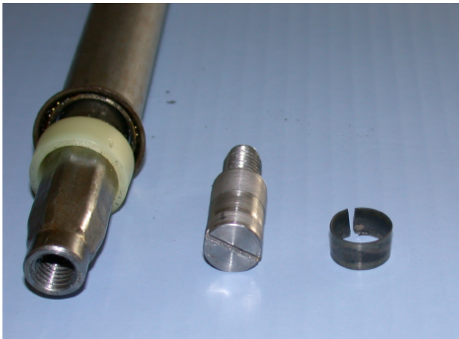
Figure 3. The Steering Column, Plain Shank Bolt, and the SMA Collar that wraps around it
