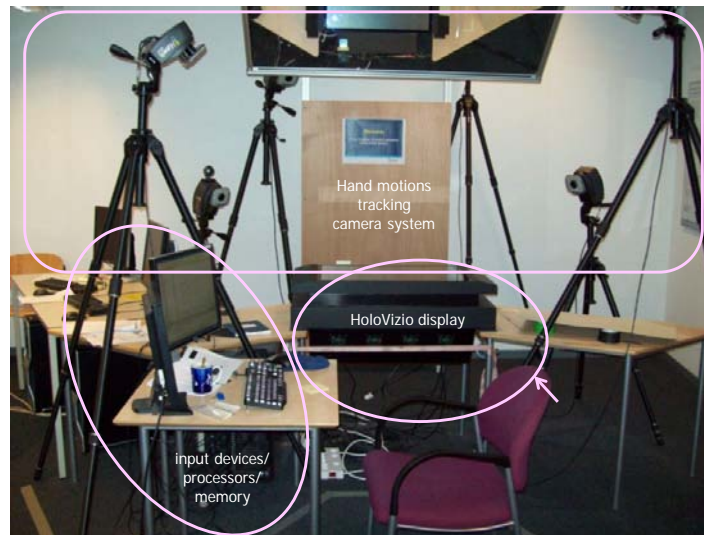
Figure 3. The selected 3D visualization technology (HoloVizio 128WD display) shown as one of the building blocks of an experimental 3D spatial product visualization system (placed like a horizontal panel on a table – it could also be constructed underneath or placed vertically just like a flat panel LCD display).
