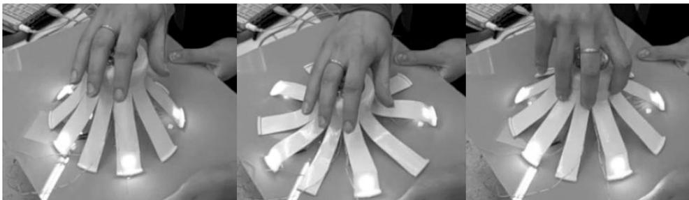
*Figure 3. This successful hack exploits a cut-up plastic cup both as a spring and as a light diffuser*
