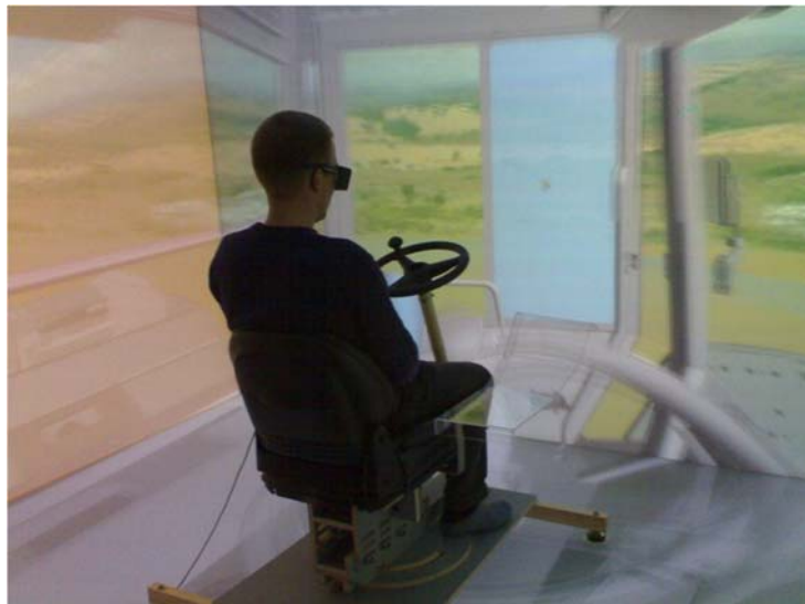
Figure 1. A static model of a machine cabin with no functionality visualized in Cave
