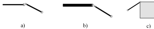
Figure 6. Connection of a line WE with another a) line WE, b) surface WE and c) volume WE.
