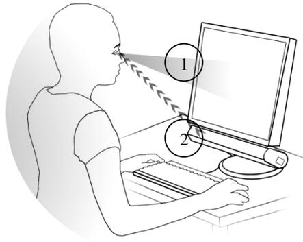
Figure 2. 1 Subject Stimulus Communication. 2 Infra-red camera recording Eye Movement.
