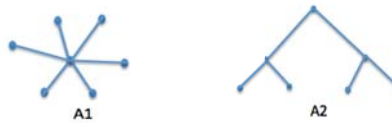
Fig. 1: Two architectures having the same number of nodes and connections but are differentiated based on their internal structure with E(A1) = 4.9 and E(A2) = 6.83 .
