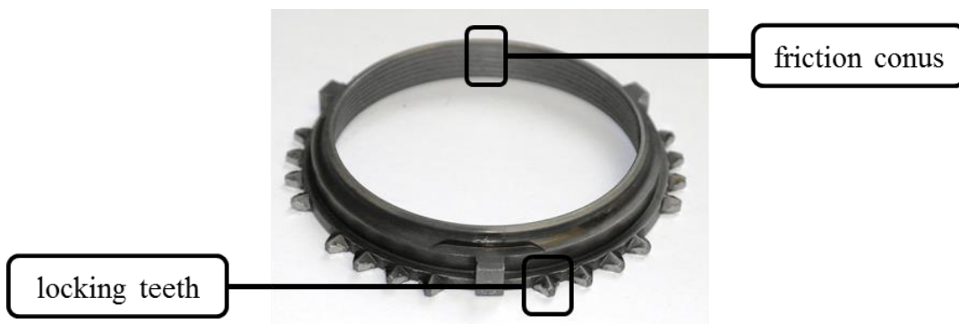
Figure 2. A synchronizer ring (produced by sintering) with exemplary SDF.
