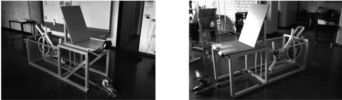
Figure 1. Modified Krogh bicycle ergometer to measure quadriceps power output
