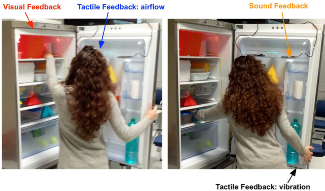
Figure 2. Two examples of tasks performed by the subject and a focus of the zones selected for placing the feedback devices (both the pictures have been made with the visual stimulus in the active mode – to make the devices visible for the picture we have removed the solutions used for hiding them).
